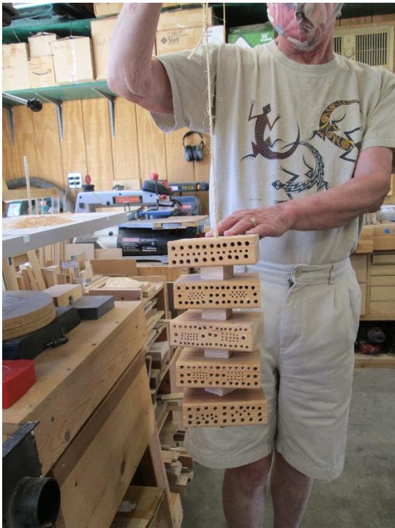
5. Added in between each 2x4 piece is a small piece of wood for design. The twine is being anchored by a small wooden toggle at the bottom block. Be creative!
