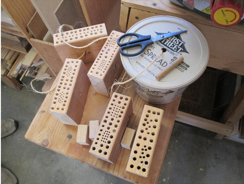
4. Here are the finished pieces with different sized holes. In the middle of each block, Harry drilled a hole through the 2x4 block perpendicular to the bee cavities. This will be for twine to string the separate block together and create a nice necklace-like design to hang.
