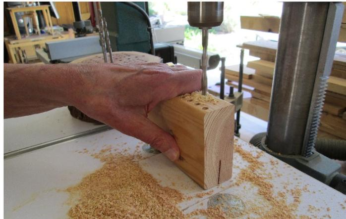
1. Here he uses a drilling machine to drill cavities for the bees in a 2x4 piece—something that is probably more commonly found around your house! He drills holes into the narrow side so the cavities for the bees to next in can be as deep as possible. Try not to make your holes too shallow—the bees will get cold!
